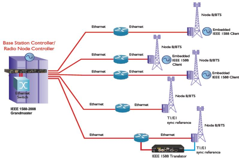
Fig. 1: IEEE-1588v2 Mobile Backhaul Implementation Example
