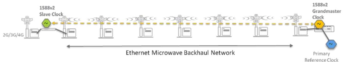
Fig. 4: Multi-Hop Linear Network Showing "bookend" Timing
