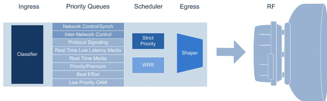
Fig. 3: Example of Microwave Traffic/QoS Management
